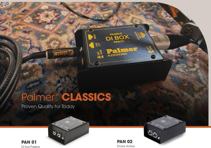
Item No. PAN01 Туре Passive Input connectors 1x 6.3 mm jack Output connectors 1x 6.3 mm jack, XLR Max. output level + 4 dBu Frequency response (±0.5 dB, relative 1 kHz) 20 Hz - 20 kHz Transformer balanced Dimensions (WxHxD) 110 x 42 x 73 mm
